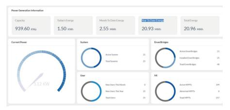
Current Power: the total generated power of all microinverters on the current day under the distributor account by the time the account is logged in to.
