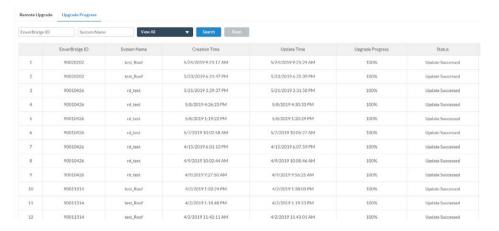
Note: The function of remote upgrade is available when EVB 202's firmware version is 004 or above, and microinverters' version is 1.7 or above.
